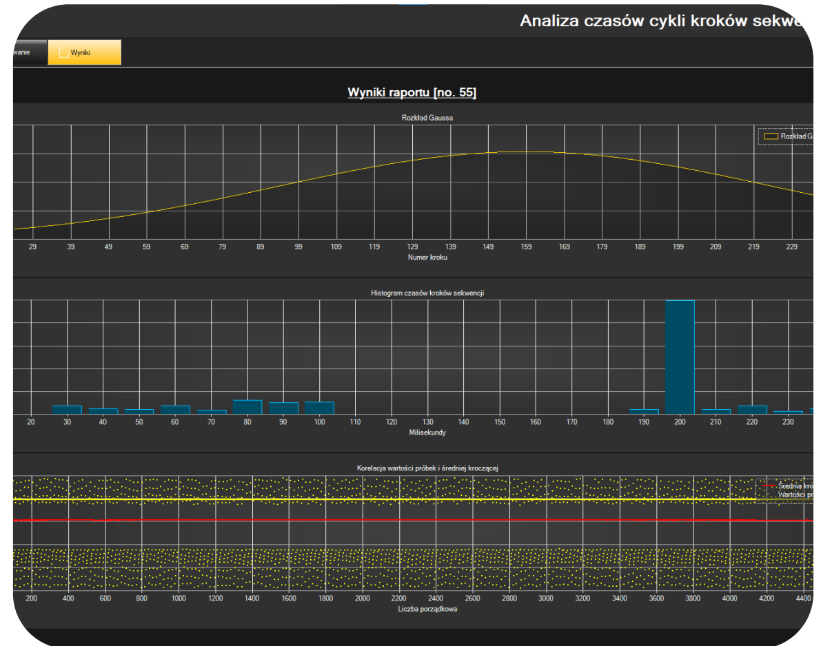
Analysis of the cycle times of the controller sequence steps. Gaussian distribution, histograms and correlations.
